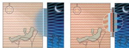
During cooler temperatures windows act like a thermal bridge allowing warm air to escape.
